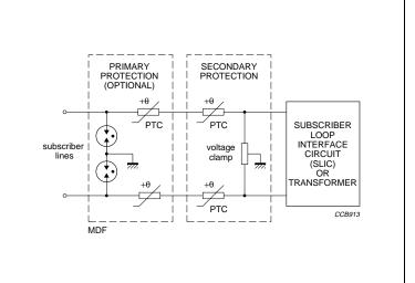
Fig. 1 Typical telephone line equipment showing where PTC thermistors can be used for overcurrent protection.
